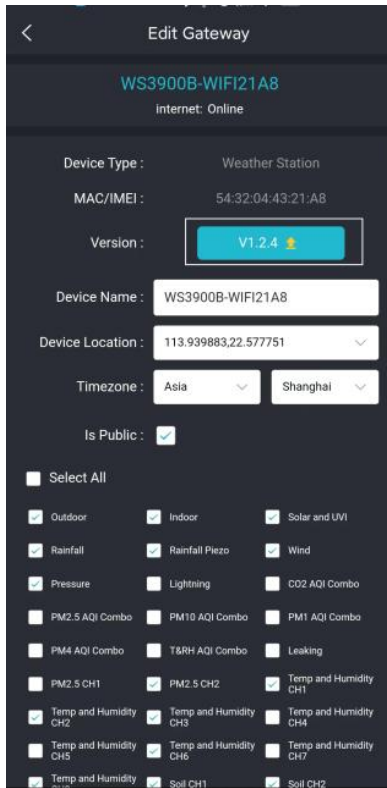
Figure 47: Firmware Upgrade on the App
